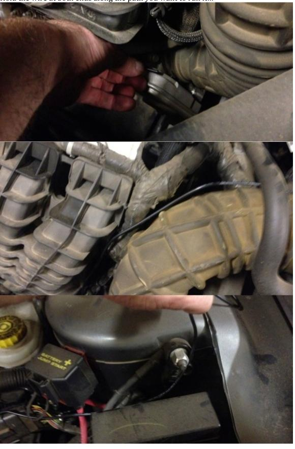
It's okay to have a little extra wire at the end; if it's too long you can tie a loop in it. If it's too short, you'll be upset. Now that you've measured, cut the wire! After that, get your wire strippers out and strip off about a quarter to 3/8 inch of insulation off each end.
