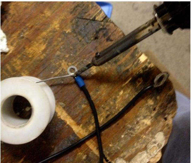
The same principle applies if you make a loop like I did on the other end; you have to get the metal of the wire hot enough for the solder to flow. Just touching the iron to them is not going to do the trick. Be careful not to overheat it though, as the wire insulation will start melting!
