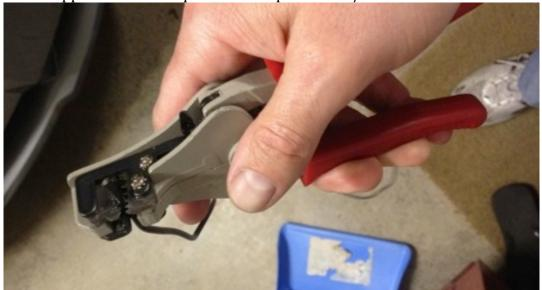
Now, slip a solderless terminal on the stripped end and squeeze it down tight. I like using the non-cutting part of a pair of dikes for this...see picture. Not the best picture, but you can see the solderless terminal squeezed between the pliers. Lineman's pliers also work
