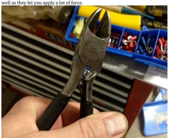
If both ends of your wire use the same size fastener/bolt, go ahead and do the other one now. The Avenger's ground point is much larger, so I elected to strip a longer portion of the other end and make a loop to match it.
