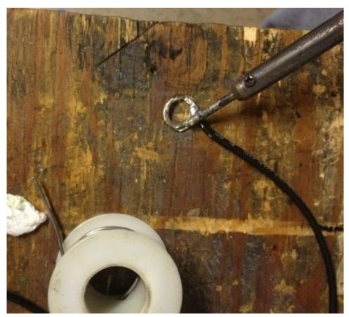
Once you have the terminals squeezed on, or in this case the loop bent to shape, plug in your soldering iron. Solder helps ensure good electrical conductivity, and makes the joint a little stronger physically. Once the soldering iron is warm enough (it will finally melt some solder if you touch it with your solder wire), press it against the metal of the wire and the solderless terminal.
