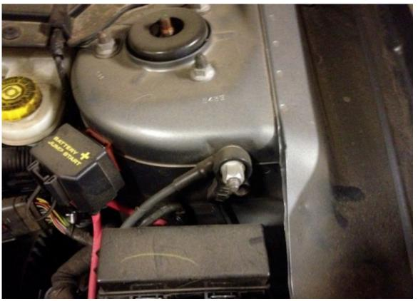
The Avenger's factory ground point is good to use; the battery is buried in the left front fender.
